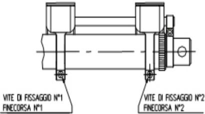
To regulate the stroke of the thrust rod according to the required values, act on micro switch 1 and 2 as follows:
