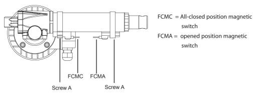
Stroke adjustoment shall be done in following steps, acting on switches "FCMA" and FCMC" as follows:
