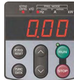
Figure 5.2 Display of the LED Monitor after Power-on
