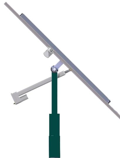
The HP5 is an electric linear actuator developed by MecVel for the photovoltaic industry. This product is able to keep a very high static load also in case of long strokes (> 500 mm), maintaining extremely low both speed and consumption (15000 N with 2 mm/s and 6 A).
