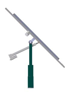
The HP5 is an electric linear actuator developed by MecVel for the photovoltaic industry. This product is able to keep a very high static load also in case of long strokes (> 500 mm), maintaining extremely low both speed and consumption (15000 N with 2 mm/s and 6 A).
