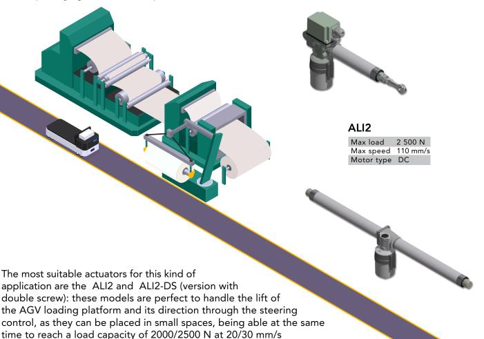
In picking and storageing phases of packed goods, electric linear actuators operate inside **cobots**, **motorized arms**, **AGVs**, **AMRs and mobile robots** in general. Movements are mainly related to the steering and the height calibration of the loading platform according to the kind and the number of packs to be transported and placed in the warehouse.
