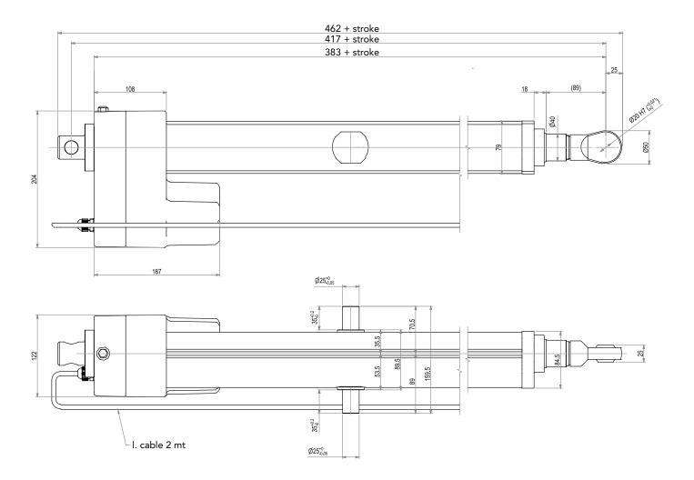
The pivots position can be arranged to the customer's needs. Contact MecVel's staff for more information.
