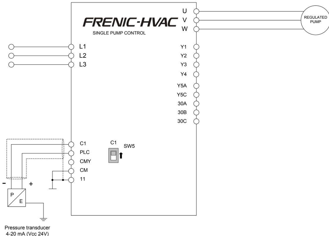
Figure 1.1: control schematic for a single pump
