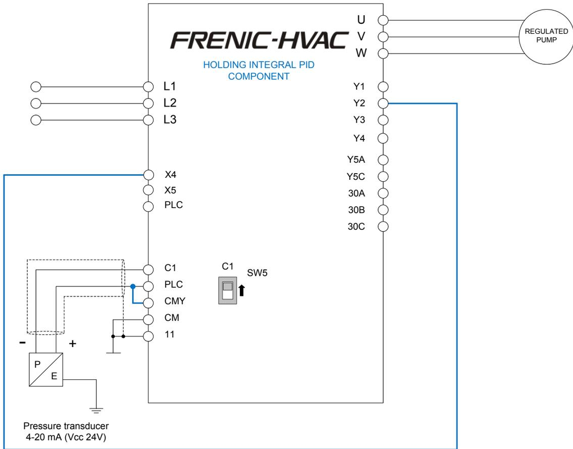
Figure 3.4: Pump control schematic for holding PID Integral component when pump is in sleep mode
