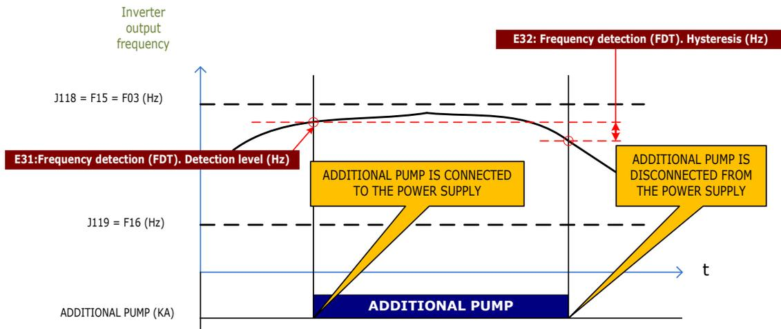
Figure 2.2: Additional pump's connection/disconnection time diagram
