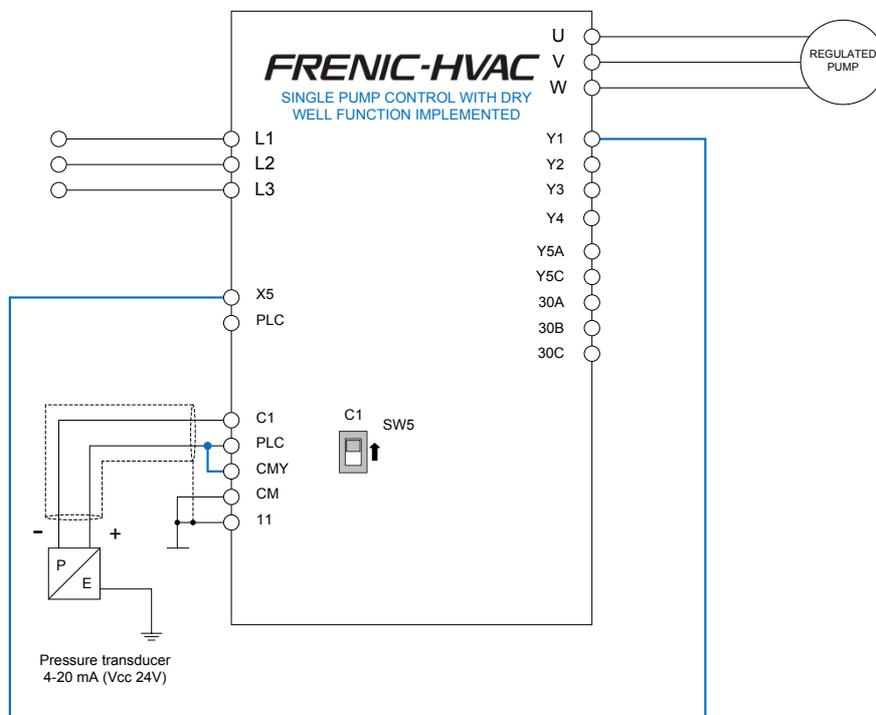
Figure 3.1: Pump control schematic for Dry well function
