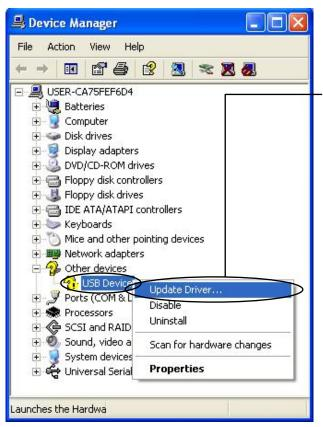
From the Start menu, select Control Panel | System | Hardware | Device Manager to open Device Manager as shown at left.
