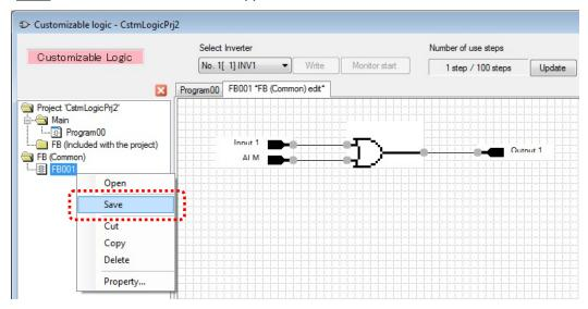
If the function block (common) is succeeded to store, the function block symbol appears in the toolbox "FB" tab.
