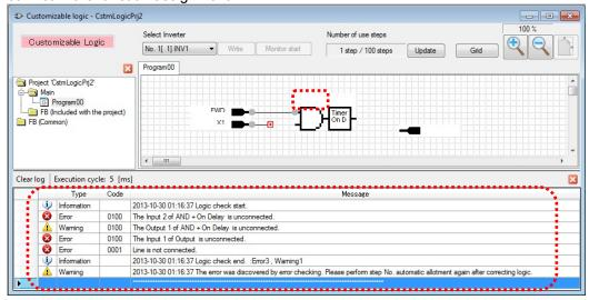
Double-clicking an error or a warning line shown in message window makes the mouse pointer jump to the relevant symbol.
