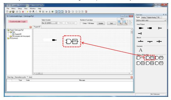
Note The execution order of the functions is determined by the layout position. Refer to Section 2.4.5 "Assigning Step Numbers".
