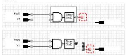
When the connection is succeeded, the red box at the end of the wire connection changes to a black box.
