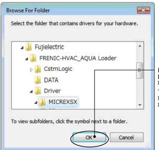
In the folder in which FRENIC HVAC/AQUA Loader has been installed, select \( \frac{4}{2}\)Driver\( \frac{4}{2}\)MICREXSX and then click \( \frac{0}{6}\)K. The default folder is C: \( \frac{4}{2}\)Fuji Electric
