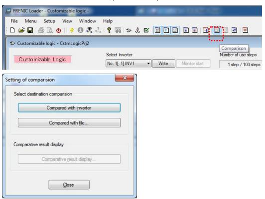
The comparison results shows inverter function codes which does not match, and it also can be saved in CSV format.
