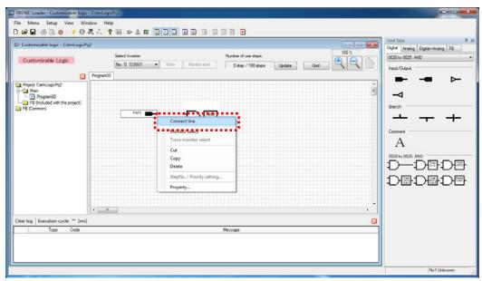
Wire connection appears. Put the cursor on the red box at the end of the wire connection, and then move the red box to the target function symbol with holding down the left button of the mouse.
