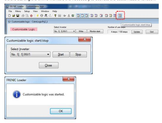
The online monitor starts after the customizable functions are executed in the inverter.
