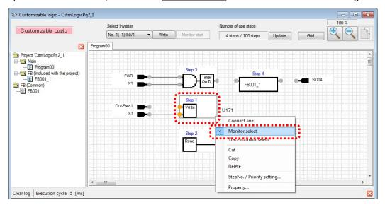
Before starting the online monitor, it is necessary to activate the customizable function.
