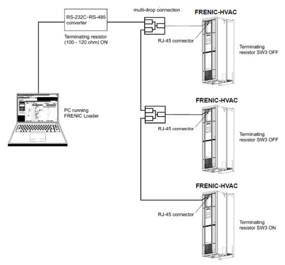
Figure 1.2.3.1. RS-485 Multi-drop Network (RJ45 connector connections)
