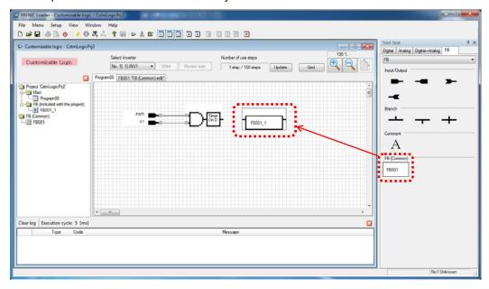
By laying out "FB001\_1", "FB001\_1" is added to the tree view under target project. By then double-clicking, a tab for editing "FB001\_1" appears.
