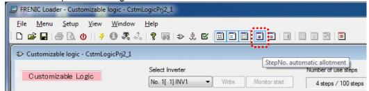
The step numbers are only available to assign if no errors have occurred after the function check.
