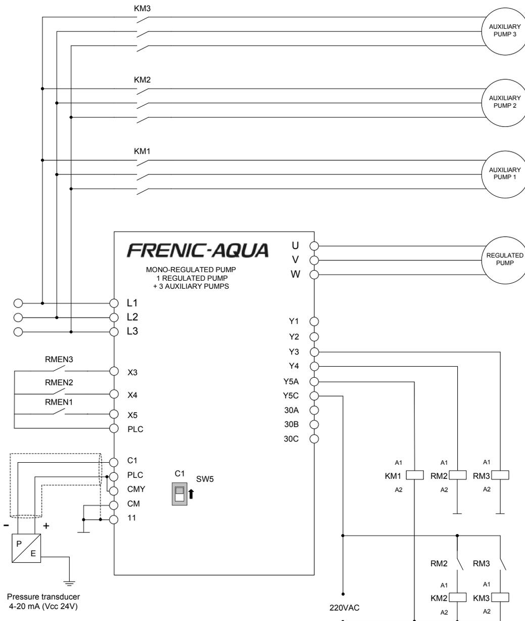
Figure 2.2: Schematic of a mono-regulated pump control with 1 regulated pump + 3 auxiliary pumps with external relays.
