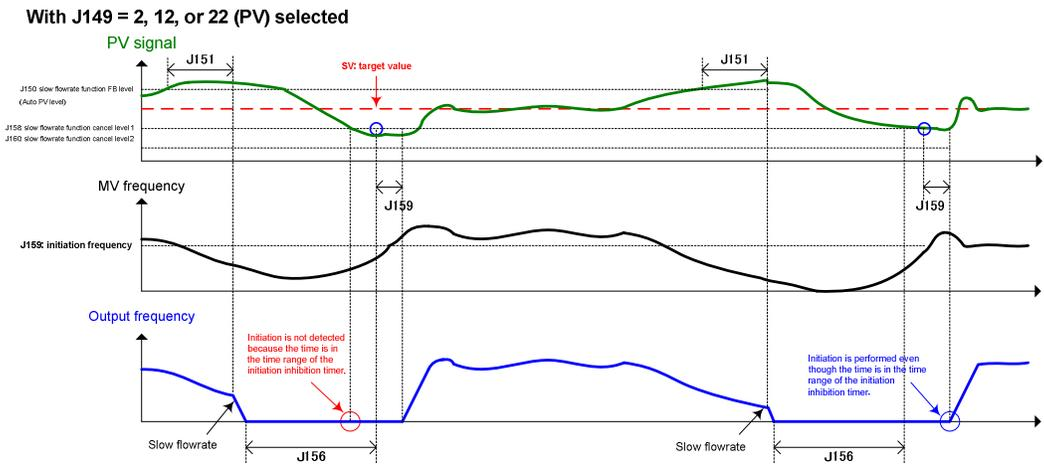
Figure 1.3: Speed control behaviour while sleep and wake-up functions are enabled and J14=2, 12 or 22.
