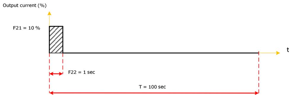
Figure 6.2: Output current when Dew Condensation prevention function is enabled
