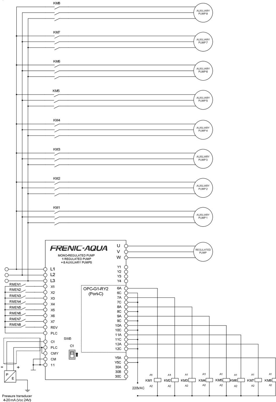
Figure 2.6: Schematic for a mono-regulated pump control with 1 regulated pump + 8 auxiliary pumps
