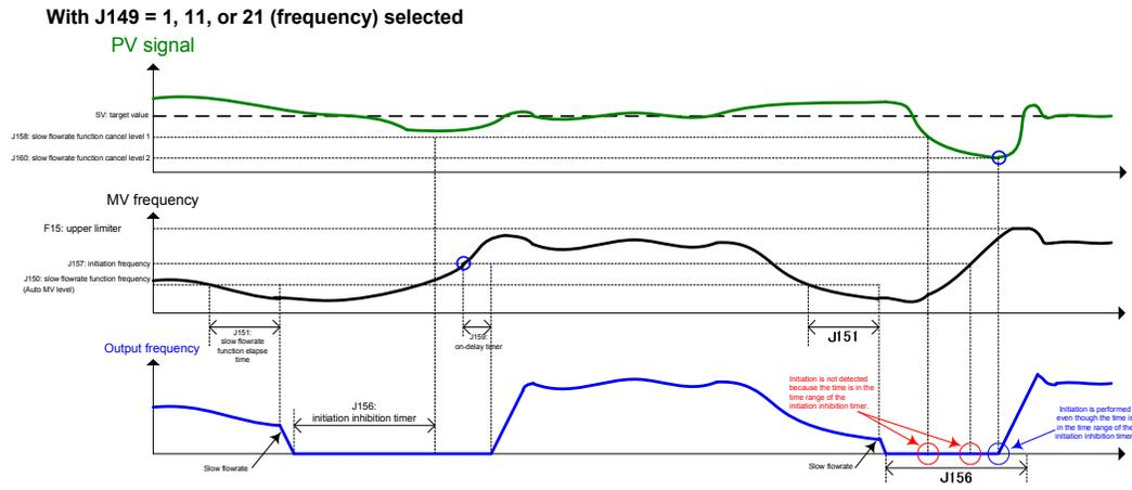
Figure 1.2: Speed control behaviour while sleep and wake-up functions are enabled and J14=1, 11 or 21.
