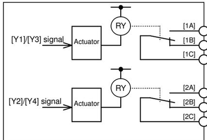
Figure 9.1 Internal Diagram OPC-G1-RY
