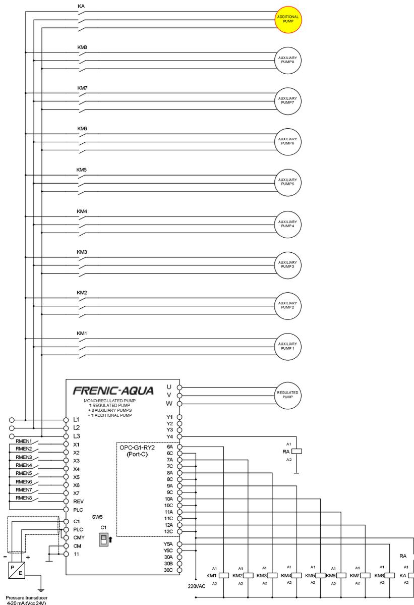
Figure 3.1: Schematic for a mono-regulated pump control with 1 regulated pump + 8 auxiliary pumps + 1 additional pump
