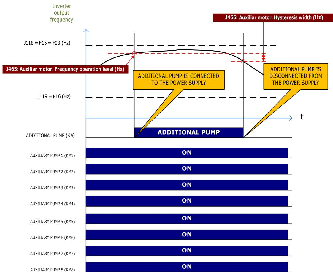
Figure 3.2: Additional pump's connection/disconnection diagram if all the auxiliary pumps are enabled
