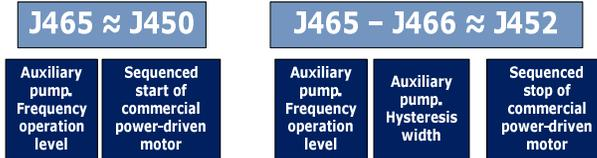
With this topology, it may be necessary to extend the disconnection time of the motor from the commercial power supply (J453), to prevent that the additional and the regulated pumps could be disconnected at the same time. That is, the additional pump must be the first one to be disconnected, and then the regulated pump, but never at the same time.
