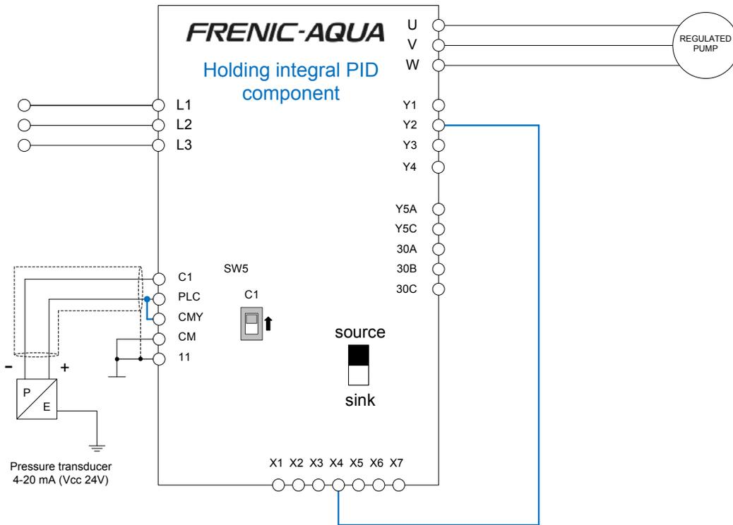
Figure 6.3: Pump control schematic for holding PID Integral component when pump is in sleep mode
