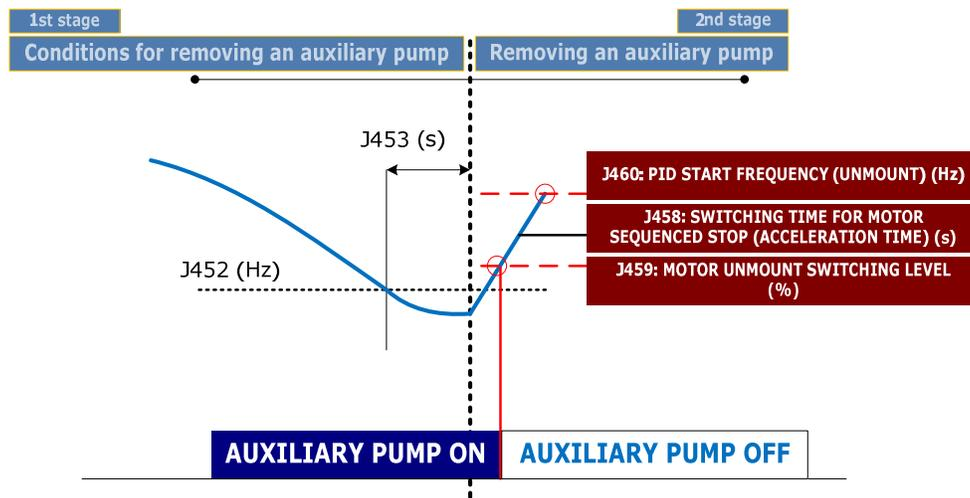
Figure 2.9: Disconnection of an auxiliary pump
