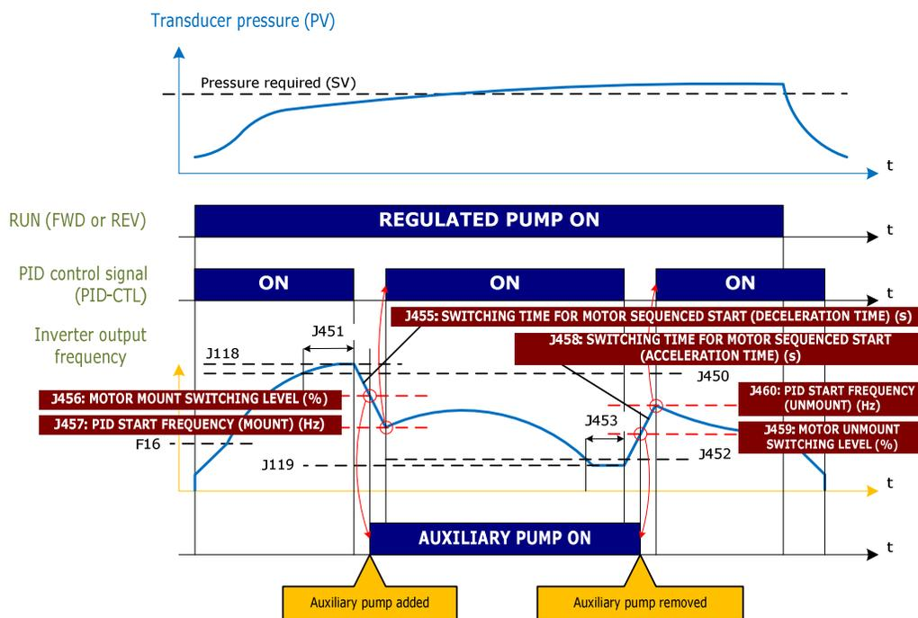
Figure 2.7: Speed pattern with mono-regulated pump control. The Auxiliary pump is connected and disconnected
