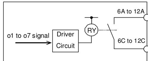
Figure 9.2 Internal Diagram OPC-G1-RY2
