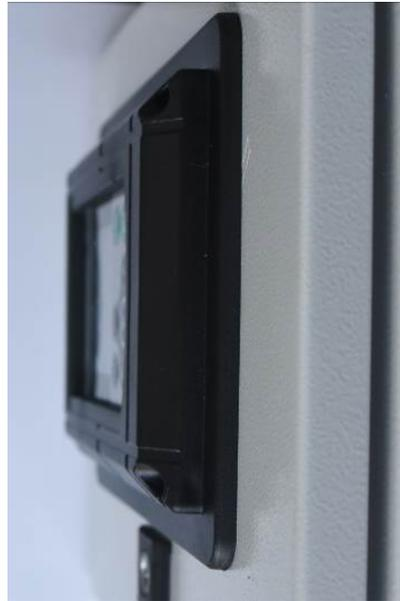
6b. Gasket compressed when fastened
