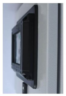
6b. Gasket compressed when fastened
