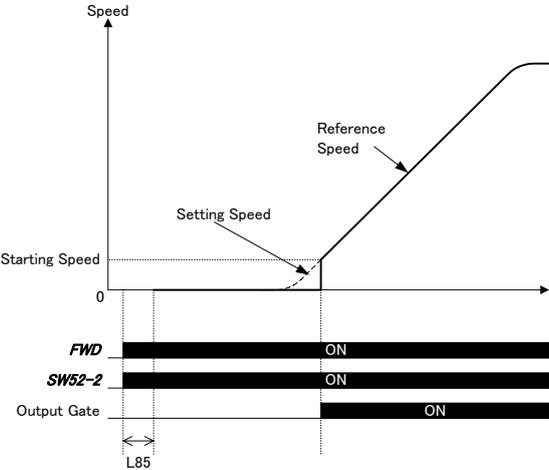
**F25****Stop Speed****H66 (Stop Speed, Detection method)
