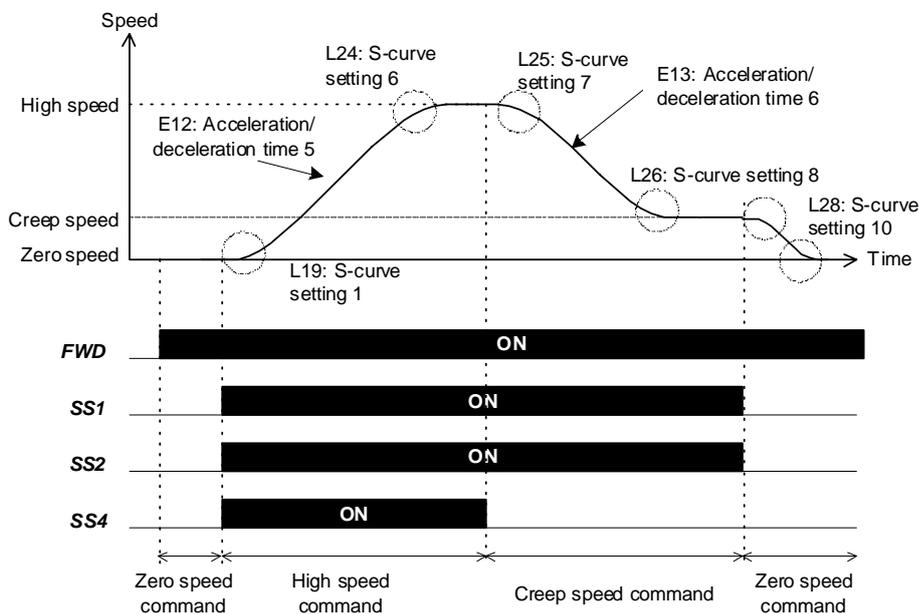
**When you give the instruction in the creep velocity while accelerating to the high speed.**
