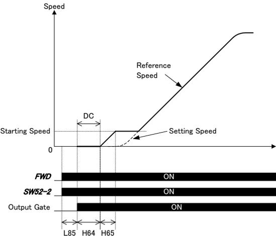
(iii) When an analog speed command (Reversible) is enabled (F01 = 2)
