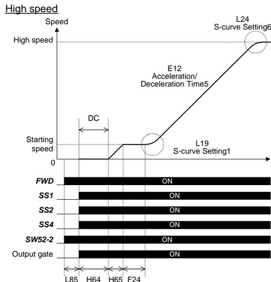
(ii) When an analog speed command (Not reversible) is enabled (F01 = 1)
