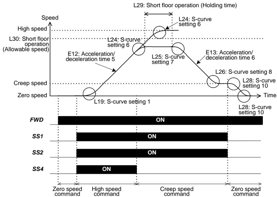
**In case of Reference speed (final) > Allowable speed (L30) and Holding time (L29) ≠ 0.00 when a deceleration command is entered**
