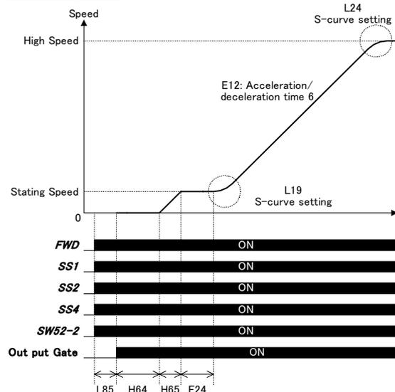
**Note** If the stop speed is specified exceeding the starting speed, the inverter does not activate a soft start as long as the reference speed (pre-ramp) does not exceed the stop speed.
