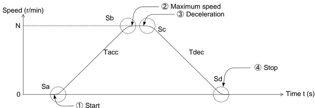
The elevator cage moves by distance "L" calculated by equations 1 and 2 when the elevator decelerates from speed "N" during deceleration period "Tdec" within S-curve zone from "Sc" to "Sd," provided that no speed error exists in inverter control. The deceleration point, therefore, should be distance "L" or more before the stop position.
