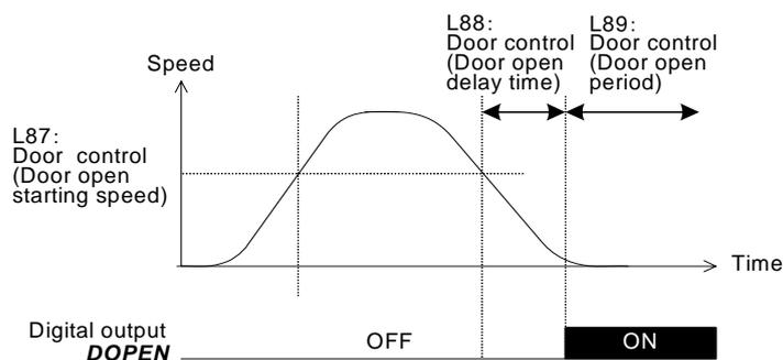
Increasing the reference speed (final) above the speed (L87) with the *DOPEN* being OFF activates the *DOPEN* ON process judgment. If the reference speed (final) does not exceed the speed (L87), the L88 and L89 specifications will be ignored so that the *DOPEN* will be kept OFF.
