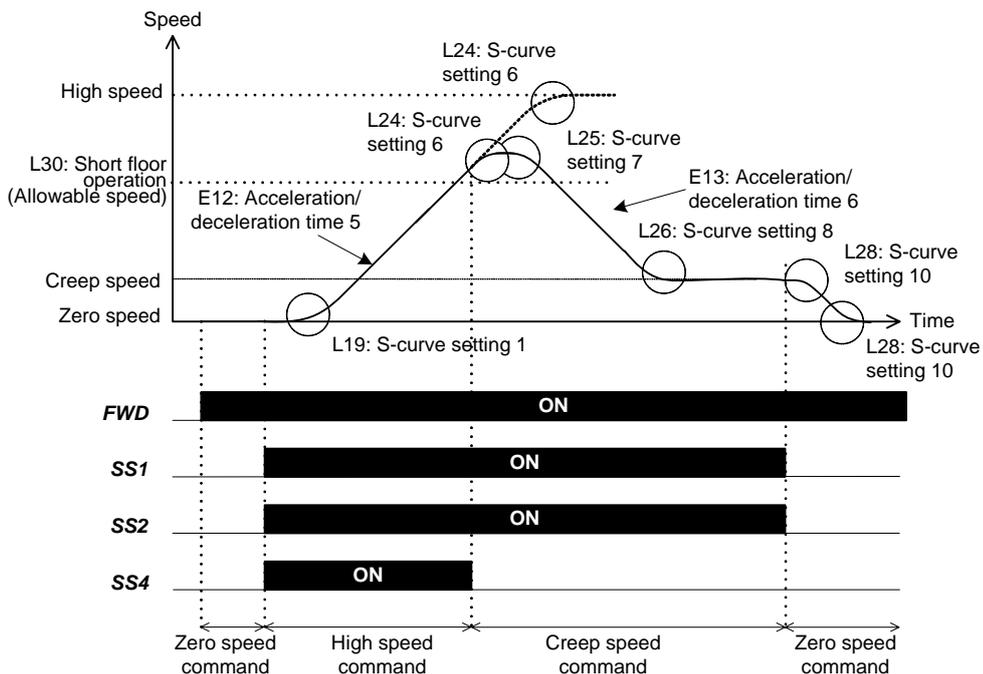
**In case of Reference speed (final) > Allowable speed (L30) and Holding time (L29) = 0.00 when a deceleration command is entered**
