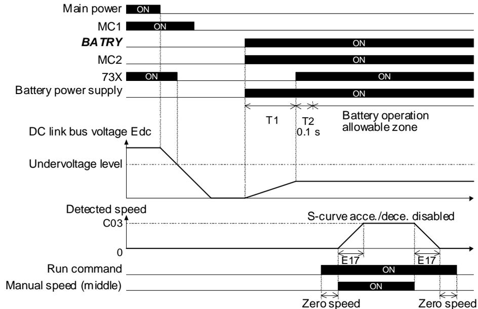
The time of  $T1$  changes depending on the voltage and capacity. Refer to the delay time of specification (4).
