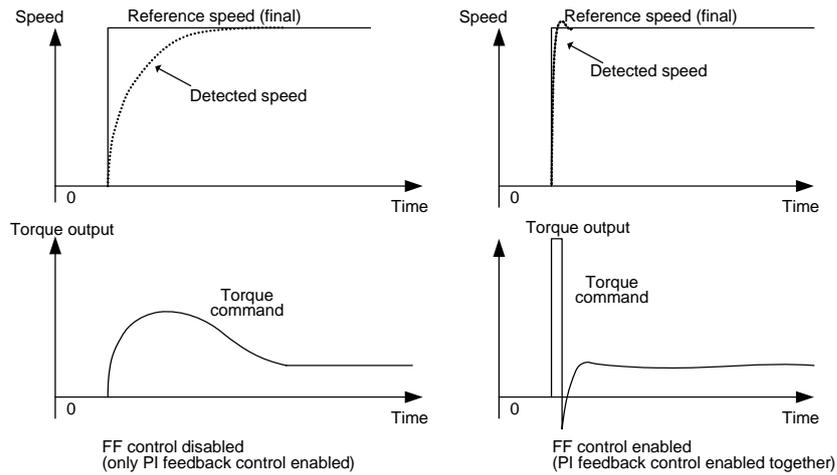
The effect above can be obtained also by adjusting the P and I constants to speed up the response, but it involves any demerits such as resonance of machinery and vibration noise.
