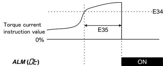
In case of vector control with PG for synchronous motor, the motor torque current is roughly proportional to the output current of the motor. But in case of vector control with PG for asynchronous motor it is not proportional to the output current of the motor.
