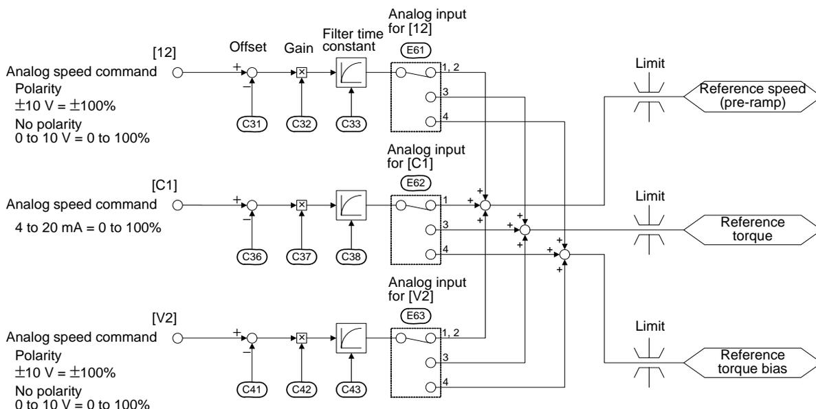
Simplified Block Diagram of Analog Inputs
