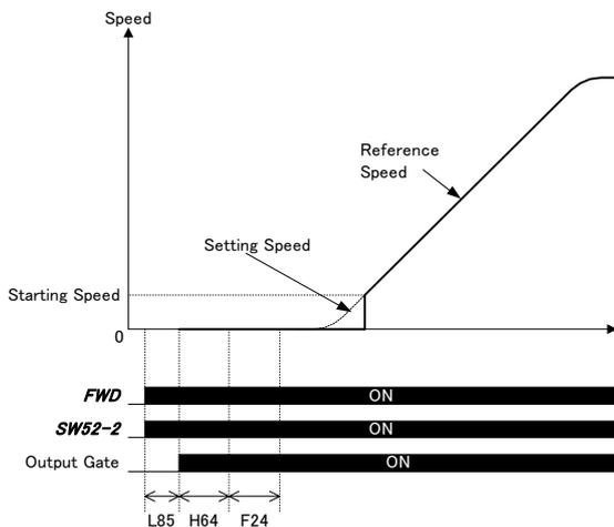
**Note** If the stop speed is specified exceeding the starting speed, the inverter does not start acceleration to the reference speed (pre-ramp) as long as the reference speed (pre-ramp) does not exceed the stop speed.
