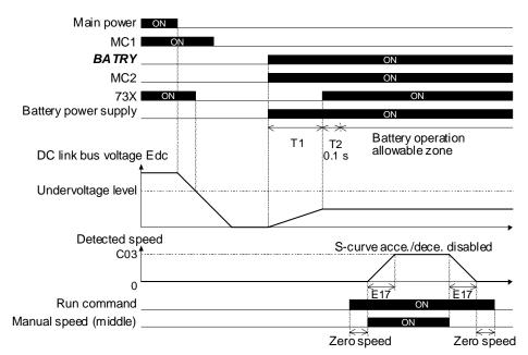
The time of T1 changes depending on the voltage and capacity. Refer to the delay time of specification (4).
