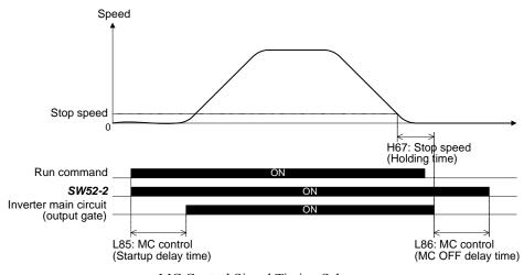
MC Control Signal Timing Scheme
