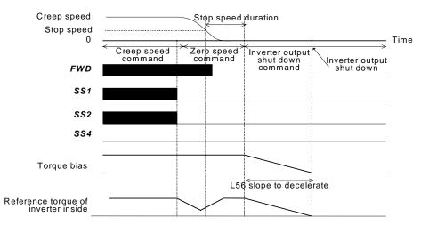
Reference Torque End Sequence in Speed Control
