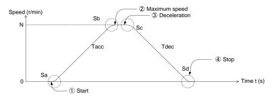
The elevator cage moves by distance "L" calculated by equations 1 and 2 when the elevator decelerates from speed "N" during deceleration period "Tdec" within S-curve zone from "Sc" to "Sd," provided that no speed error exists in inverter control. The deceleration point, therefore, should be distance "L" or more before the stop position.
