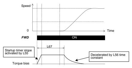
Reference Torque End Sequence in Torque Control
