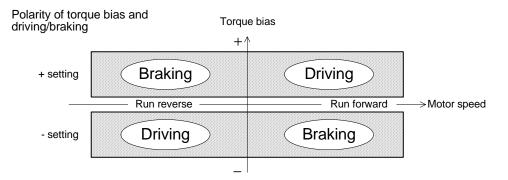
In the figure shown above, when viewed from the motor shaft, the counterclockwise rotation means the forward direction, and the clockwise rotation, the reverse direction. The torque bias (+) is a forward direction torque.
