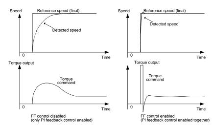
The effect above can be obtained also by adjusting the P and I constants to speed up the response, but it involves any demerits such as resonance of machinery and vibration noise.
