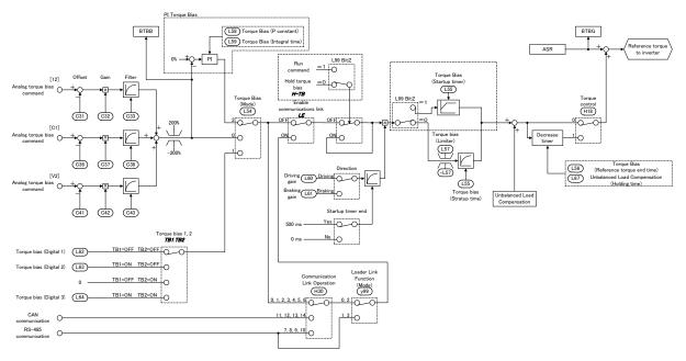
Block Diagram of Torque Bias Generator
