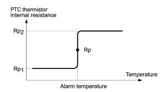
Suppose that the resistance of PTC thermistor at alarm temperature Rp, the detection (voltage) level  $V_{v2}$  is calculated by the equation below. Set the result  $V_{v2}$  to function code H27.
