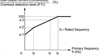
Cooling Characteristics of Motor Equipped with a Self-cooling Fan
