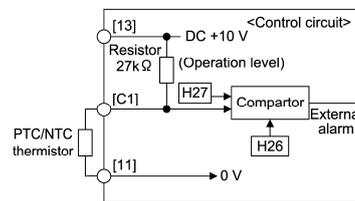
Figure 3.4 Internal Circuit Diagram (SW5 Selecting PTC/NTC)
