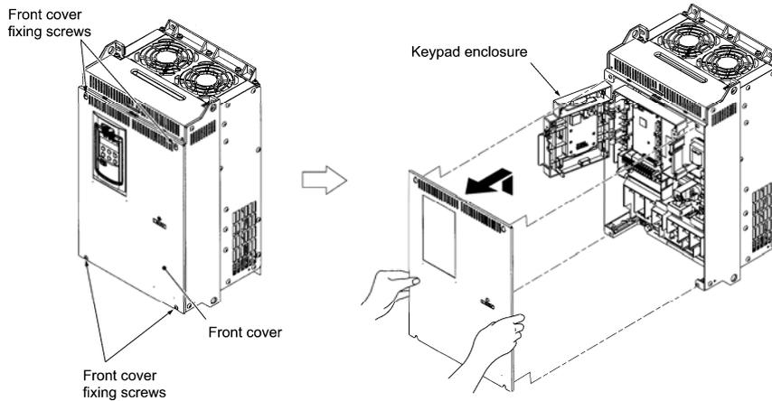
Tightening torque: 1.8 N·m (M4)
