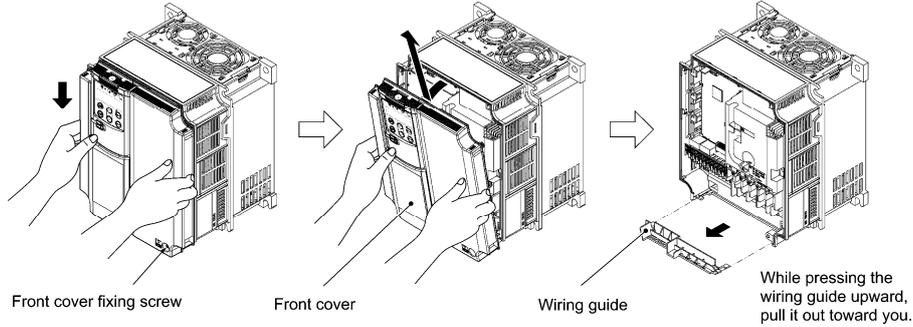
Figure 3.1 Removing the Front Cover and the Wiring Guide
