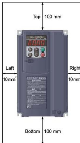
\* For the inverters with a capacity of 1.5 kW or below and 30 kW or above, maintain 50 mm clearance to the right and left sides, 100 mm to the front.
