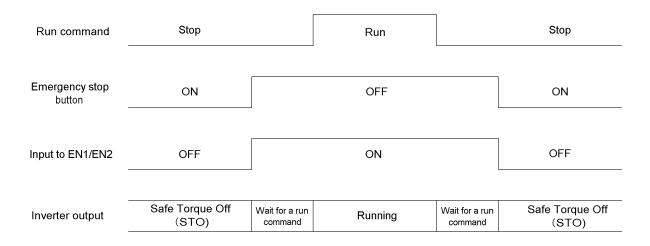
Figure 9.7 Inverter Output State when the Emergency Stop Button is turned OFF with the inverter being stopped
