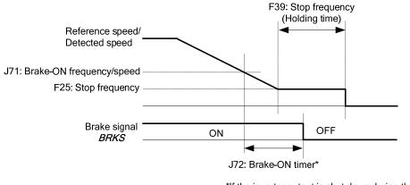
\*If the inverter output is shut down during the timer period specified by J72, the inverter ignores the timer count and activates the brake.
