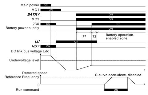
Battery Operation Timing Diagram
