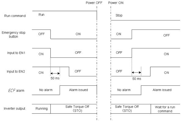
Figure 9.9 ELF Alarm (Caused by Logic Discrepancy) and Inverter Output State
