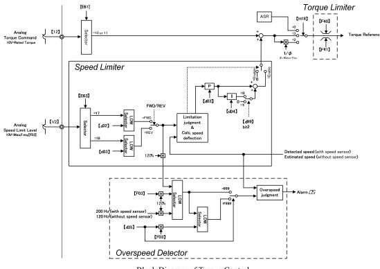
Block Diagram of Torque Control
