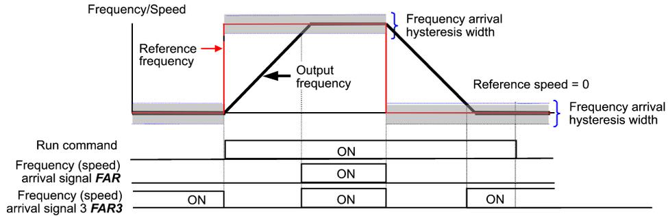
**E31, E32 Frequency Detection (Level and Hysteresis width)** E36, E54 (Frequency Detection 2 and 3 (Level))
