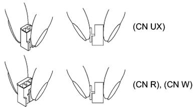
**Note** To remove each of the jumpers, pinch its upper side between your fingers, unlock its fastener, and pull it up.
