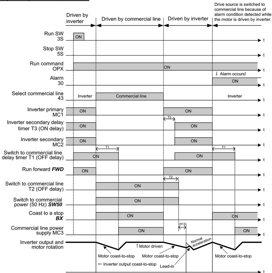
**Tip** Alternatively, you may use the integrated sequence by which some of the actions above are automatically performed by the inverter itself. For details, refer to the description of *ISW50* and *ISW60*.
