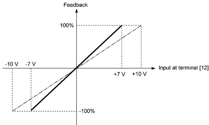
Example 2. When the output level of the external sensor is 0 to 10 VDC:
