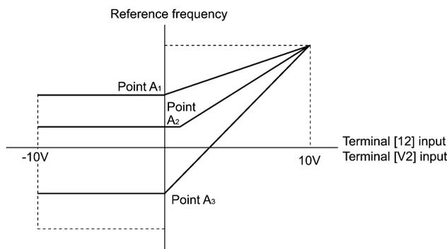
**Note** A reference frequency can be specified not only with the frequency (Hz) but also with other menu items, depending on the setting of function code E48 (= 3 to 5, or 7).
