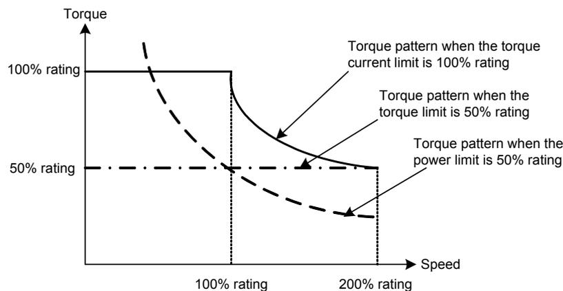
■ Torque Limiter (Target quadrants) (H75)
