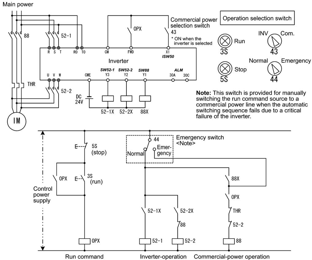
3) Sequence with an emergency switching function --Part 2 (Automatic switching by the alarm output issued by the inverter)
