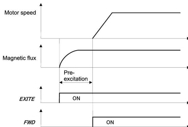
**Note** In V/f control (including auto torque boost and torque vector), pre-excitation is disabled. Use the DC braking or the starting frequency instead.
