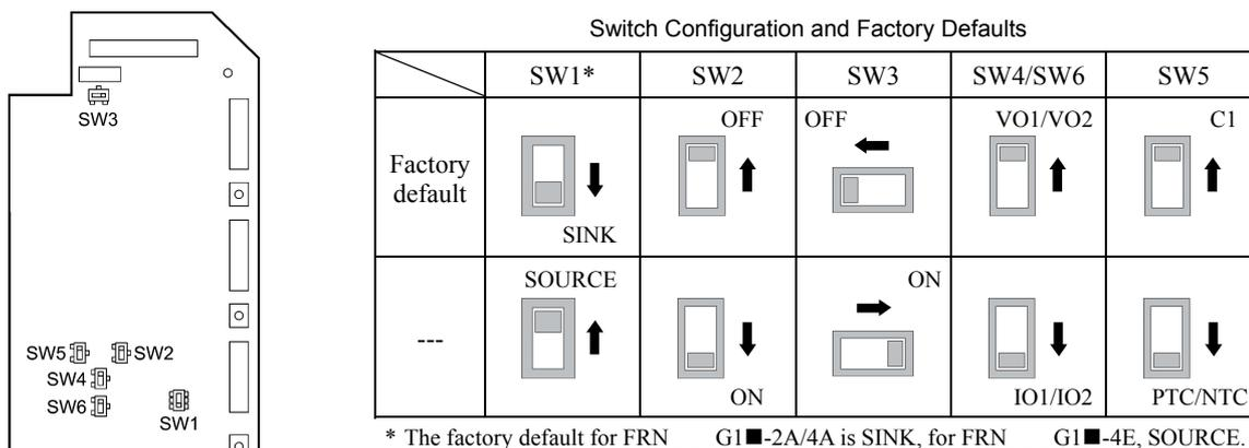
Figure 2.20 Location of the Slide Switches on the Control PCB
