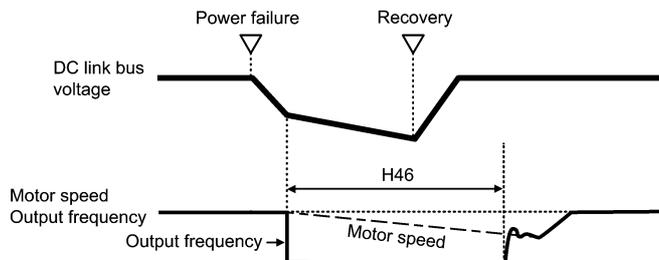
Under auto search control, the inverter searches the motor speed with the voltage applied at the motor start and the current flowing in the motor, based on the model built with the motor parameters. Therefore, the search is greatly influenced by the residual voltage in the motor.
