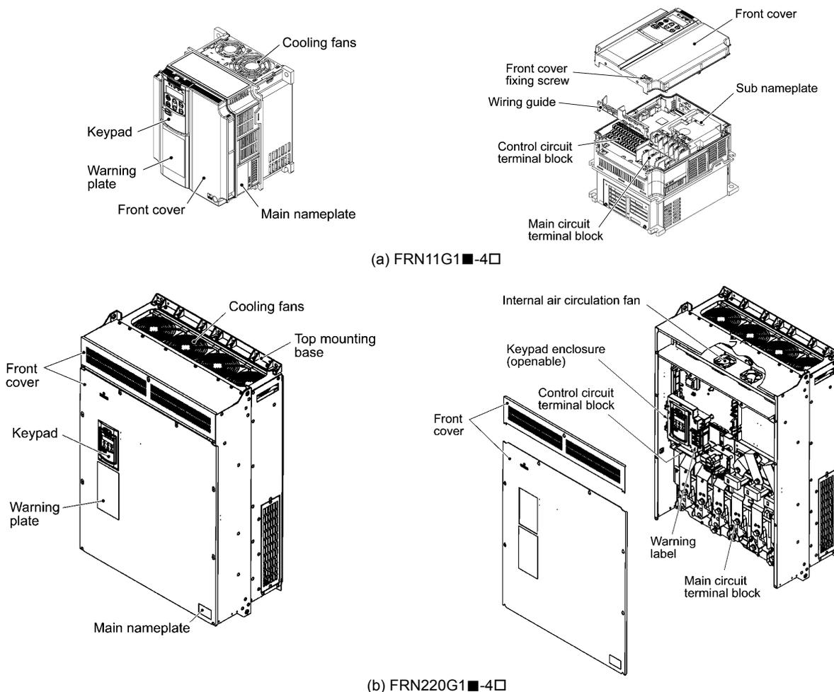
Figure 1.2 Outside and Inside Views of Inverters
