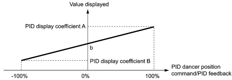
If the sensor output is unipolar, the PID dancer control operates within the range from 0 to  $+100\%$ , so virtually specify the value at  $-100\%$  as coefficient B.
