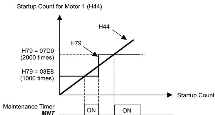
To enable this function, assign the maintenance timer signal **MNT** to one of the digital output terminals (function code data = 84).
