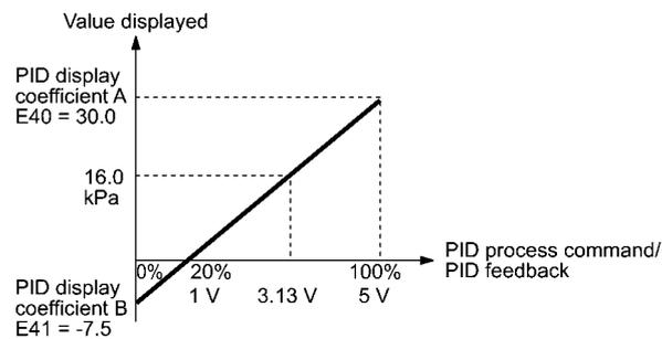
■ Display coefficients for PID dancer position command and its feedback (J01 = 3)
