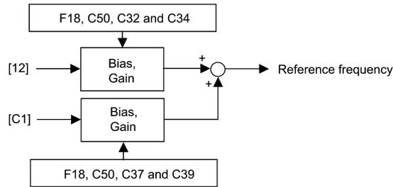
In the case of unipolar input (terminal [12] with C35 = 1, terminal [C1], terminal [V2] with C45 = 1)
