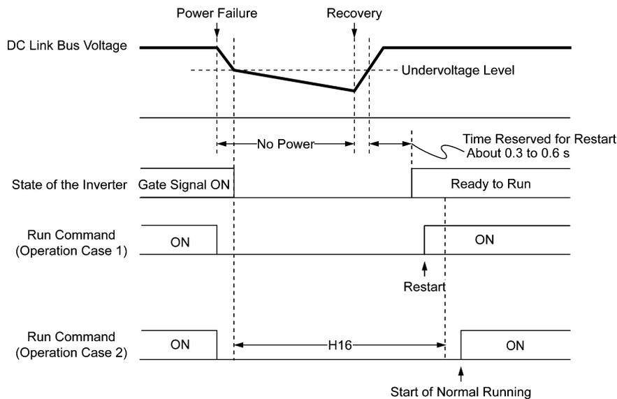
If H16 (Allowable momentary power failure time) is set to "999," restart will take place until the DC link bus voltage drops down to the allowable voltage for restart after a momentary power failure (50 V for 200 V class series and 100 V for 400 V class series). If the DC link bus voltage drops below the allowable voltage, the inverter recognizes that the power has been shut down so that it does not restart but starts (normal starting).
