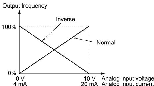
**Tip** The normal/inverse switching operation is useful for air-conditioners that require switching between cooling and heating. In cooling, the speed of the fan motor (output frequency of the inverter) is increased to lower the temperature. In heating, it is reduced to lower the temperature. This switching is realized by this *IVS* terminal command.
