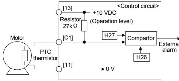
**Note** When using the terminal [C1] for PTC/NTC thermistor input, also turn SW5 on the control printed circuit board to the PTC/NTC side. For details, refer to Chapter 2, "SPECIFICATIONS."
