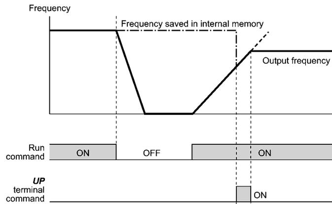
Initial frequency for the **UP/DOWN** control when the frequency command source is switched
