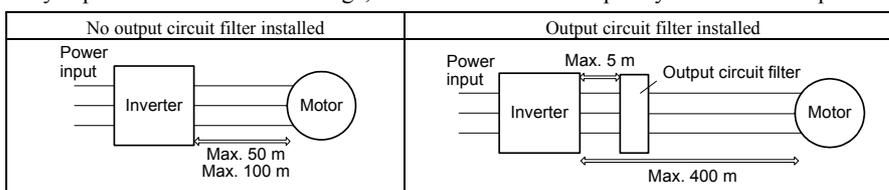
For an inverter with an output circuit filter installed, the total secondary wiring length should be 400 m or less (100 m or less under the vector control).
