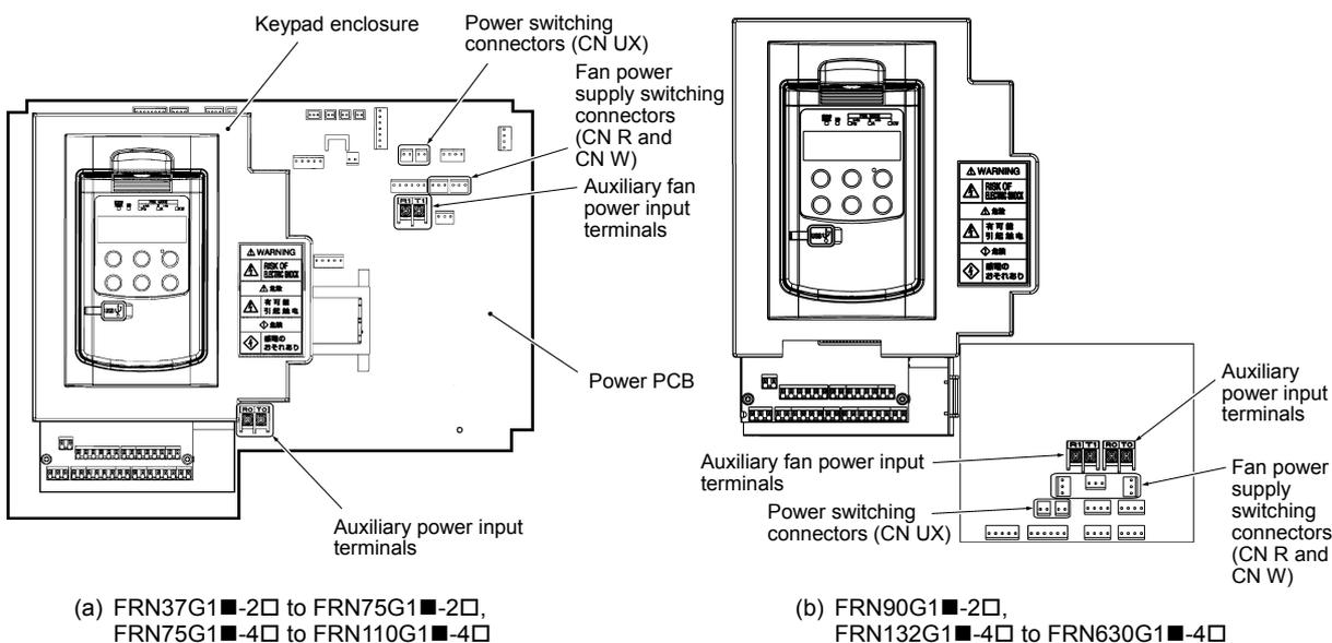
Figure 2.6 Location of Switching Connectors and Auxiliary Power Input Terminals
