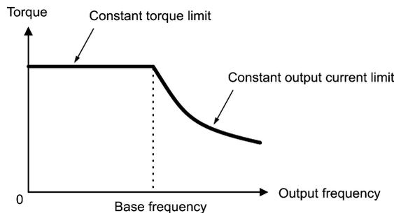
■ Torque limiter 1-1, 1-2, 2-1 and 2-2 (F40, F41, E16 and E17)
