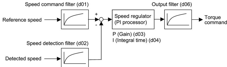
■ **Speed command filter (d01)** Data setting range: 0.000 to 5.000 (s)
