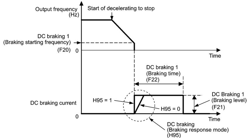
**Tip** It is also possible to use an external digital input signal as an "Enable DC braking" terminal command **DCBRK**. As long as the **DCBRK** command is ON, the inverter performs DC braking, regardless of the braking time specified by F22. (Refer to E01 through E07, data =13.)
