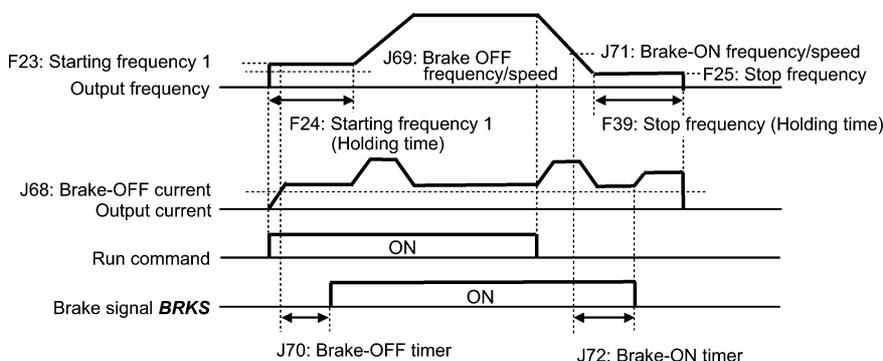
Operation time chart under vector control without speed sensor
