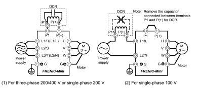
Figure 10.1 Connection Diagram of DC Reactor (DCR)
