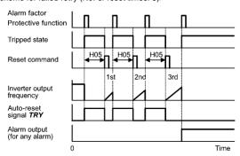
The auto-reset operation can be monitored from the external equipment by assigning the digital output signal TRY to any of the programmable output terminals [Y1] and [30A/B/C] with E20 or E27 (data = 26).
