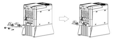
Figure 11.1 Attaching the EMC Grounding Flange
