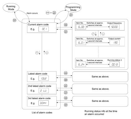
Figure 3.11 Alarm Mode Status Transition
