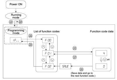
Figure 3.5 Example of Function Code Data Changing Procedure
