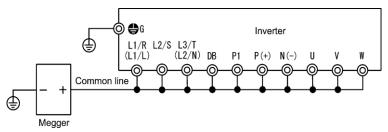
Figure 7.2 Main Circuit Terminal Connection for Megger Test
