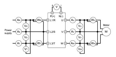
Figure 7.1 Connection of Meters
