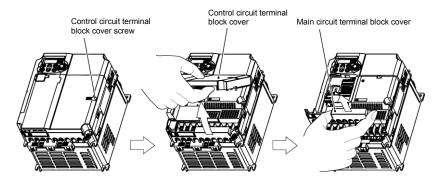
Figure 2.3 Removing the Terminal Block Covers
