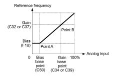
Example: Setting the bias, gain and their base points when the reference frequency 0 to 100% follows the analog input of 1 to 5 VDC to terminal [12] (in frequency command 1).
