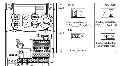
Figure 2.12 Locations of Jumper Switches and RJ-45 Connector
