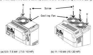
Figure 2.3 Fixing the Cooling Fans
