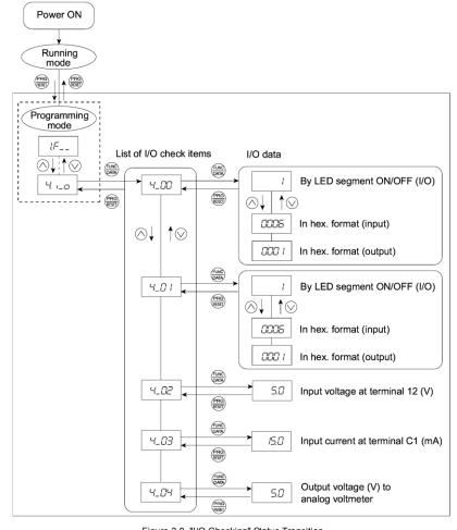
Figure 3.8 "I/O Checking" Status Transition
