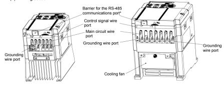
(\* When connecting the RS-485 communications cable, remove the control circuit terminal block cover and cut off the barrier provided in it using nippers.)
