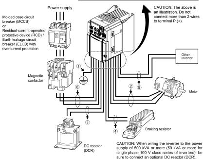
Figure 2.4 Wiring Procedure for Peripheral Equipment
